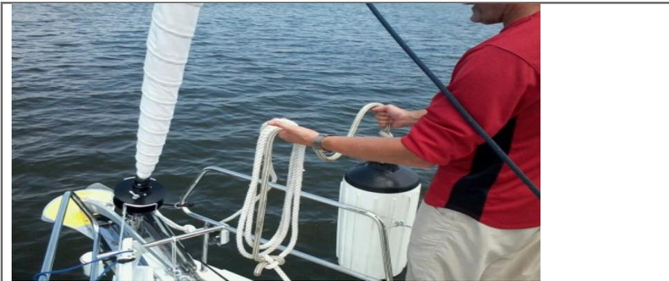
***Attach trip line to anchor, calculate length required (depth + tide + 10 feet), lead trip line outside pulpit***
