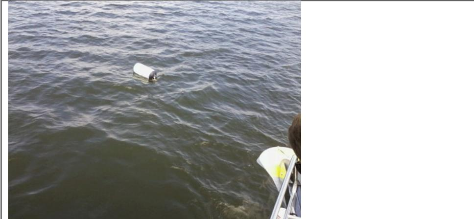
***As anchor rode is paid out, throw buoy clear to mark location of anchor - then pull buoy aboard when ready to leave***
